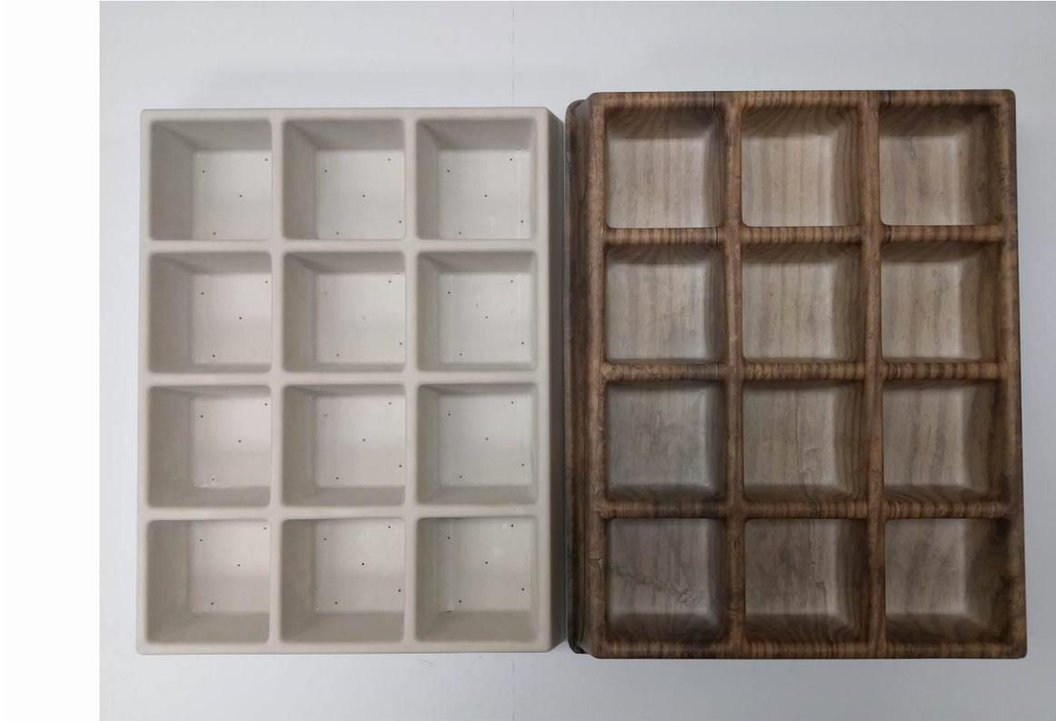
*The 3D Printed tool on the left with the thermoformed tray using a heat resistant Stretch-able ink is on the right.*
